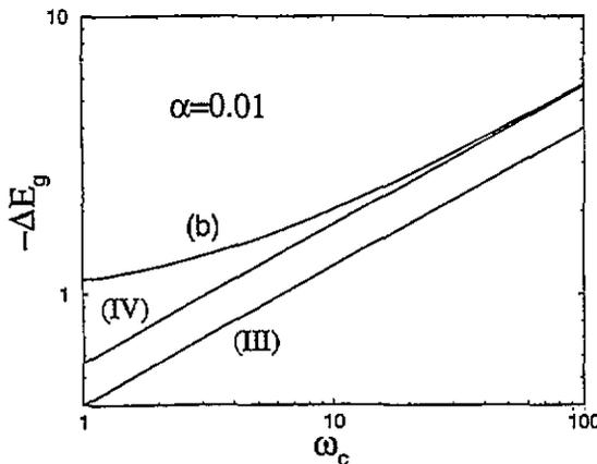
Figure 1. The asymptotic profiles for  $\Delta E_g$  in the high-field limit. Curve (b) displays the results for the improved version in the present calculation. The straight lines (III) and (IV) are the strong-coupling results plotted from equations (2) and (16), (17), respectively. The energies are expressed in terms of the free-polaron binding energy,  $(\pi/2)\alpha$ .
